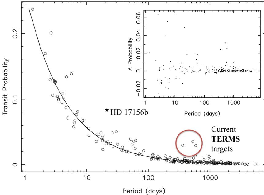
Figure 2: **TERMS:**  $P_t$  for 203 exoplanets from the catalog of Butler et al. (2006), based on their tabulated orbital parameters (open circles). The solid line shows  $P_t$  for circular orbits. Differences between  $P_t$  for circular and actual orbits are shown in insert. The three current TERMS targets (due to their inflated  $P_t$  values) are HD 156846b, HD 4113b, and HD20782b. For purposes of comparison, we assume solar/Jupiter masses and radii for the stars/planets.
